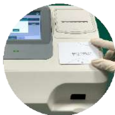
Magnetic card calibration
